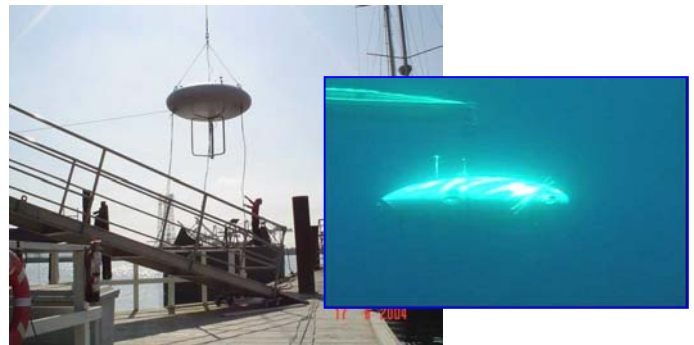
Figure 1. NAF Sea Experimentation: Photo of 3m NAF with 5 kW vertical axis-type propeller generator being positioned on its’ mooring prior to being towed and placed in 200 foot deep waters off of Santa Catalina Island, California. (Insert) Undersea photo of 1m NAF with 20 watt Wells turbine-type propeller generators, in the same location
